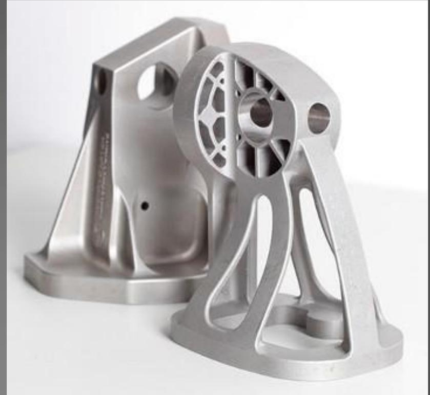
Optimized Airbus A380 bracket printed in stainless-steel (front) as a replacement for the standard cast steel bracket (rear)
